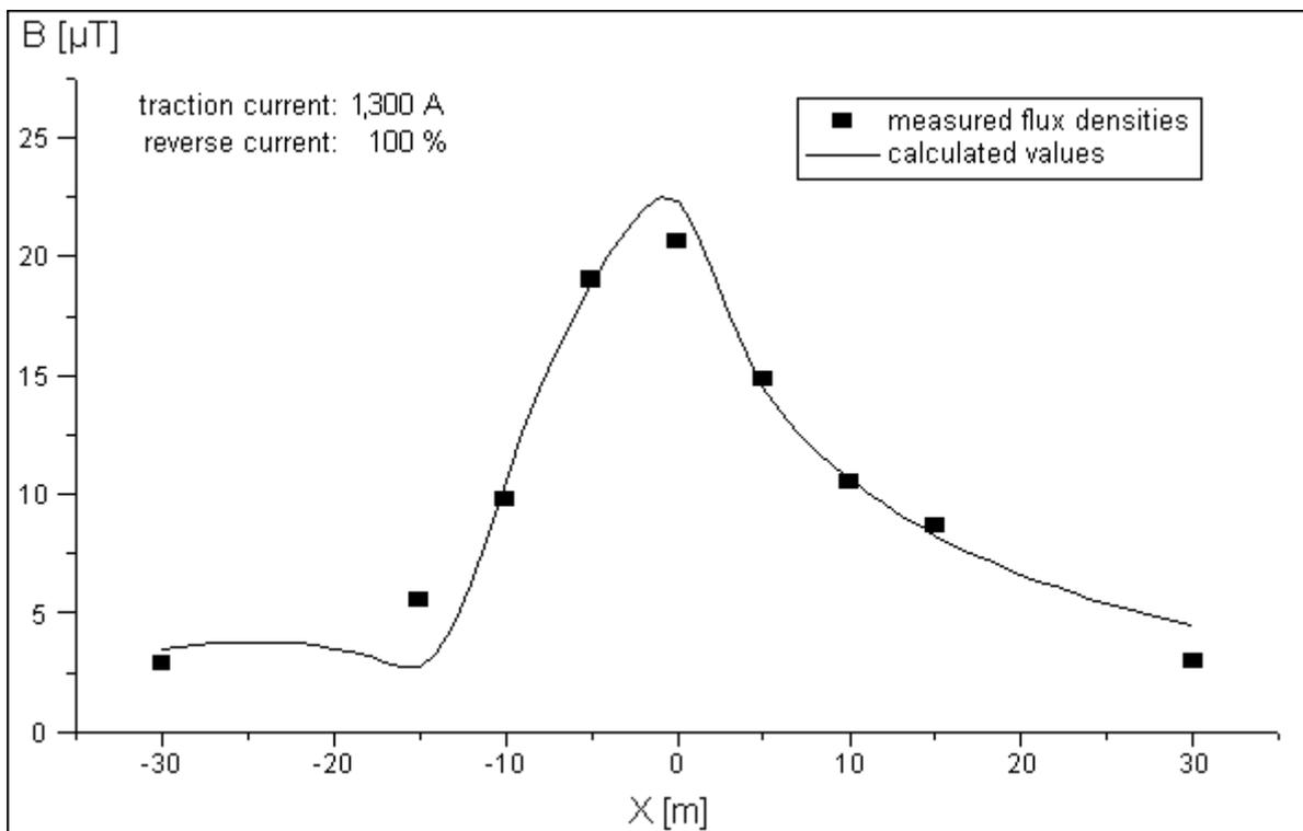
**Fig. 11: Measured and Calculated Development of the Magnetic Field under the Bridge over Knesebeckstrasse in Berlin-Charlottenburg**
