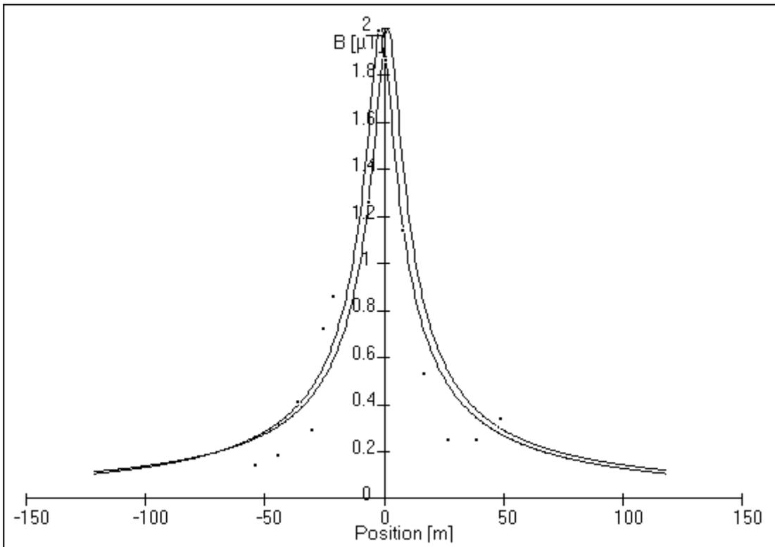
**Fig. 9: Peak Magnetic Flux Densities by the Railroad Track - Determined by Simulation**
