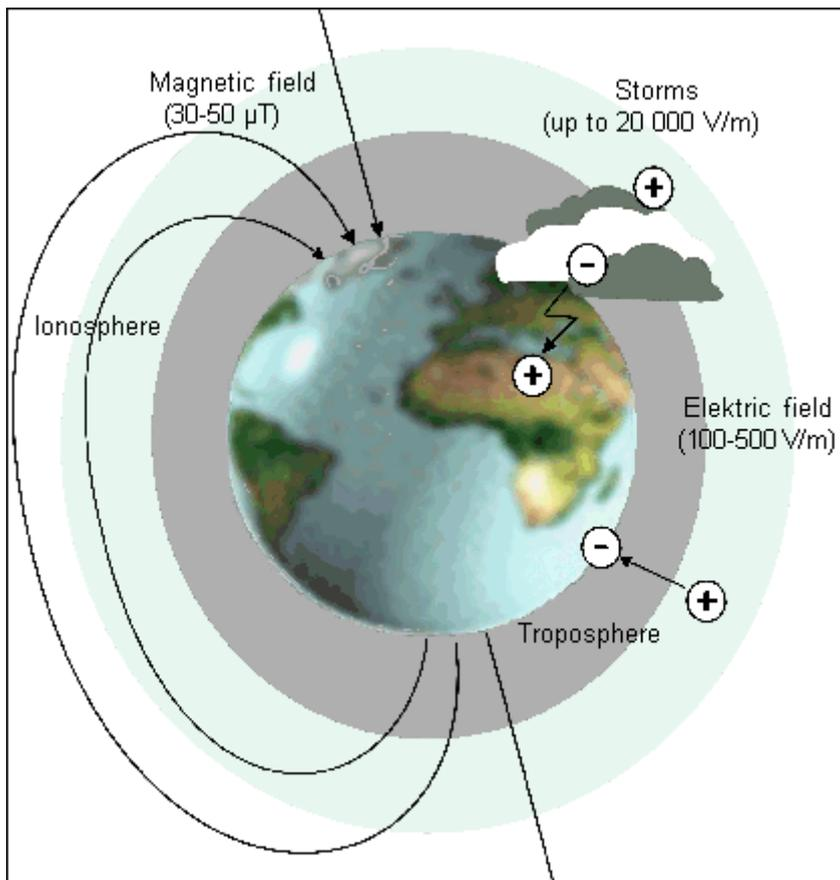
*Fig. 4: Natural Electric (Direct) and Magnetic (Constant) Fields*
