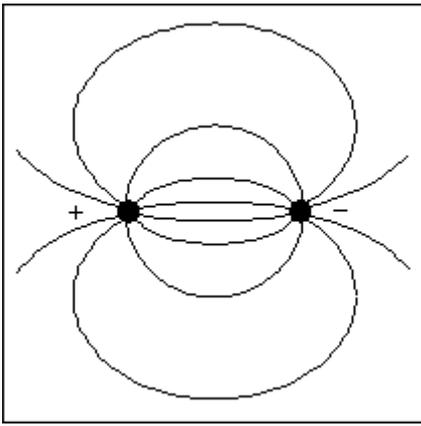
*Fig. 2: Electric Field Lines around a Double-wire Cable*
