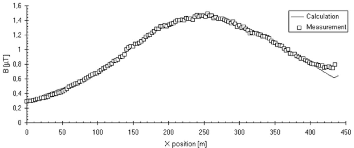
*Fig. 7: Measured and Calculated Longitudinal Profile of Magnetic Flux Density 1 m above Ground beneath an 380 kV Overhead Line. The Pylons are Situated at Positions 0 m and 440 m.*
