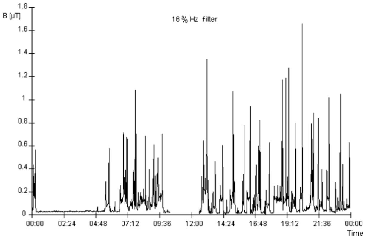
*Fig. 8: Magnetic Flux Density at 11.2 m Distance from the Railtrack in Schlüterstrasse, Berlin-Charlottenburg*
