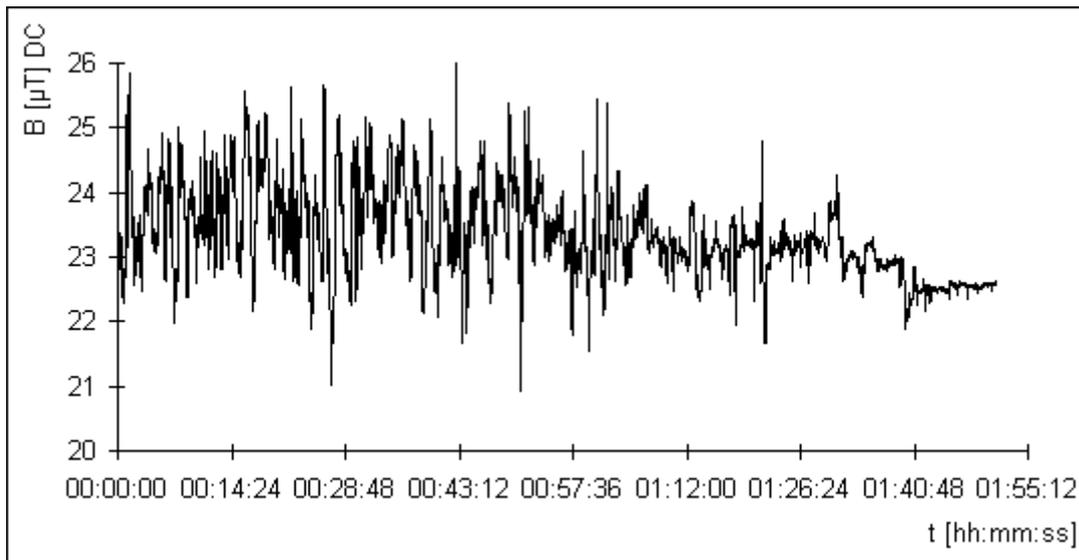
**Fig. 10: Constant Magnetic Field beneath the S-Bahn Bridge over Knesebeckstrasse by Savignyplatz during Night-time Measurement which Shows Rail Traffic Waning**
