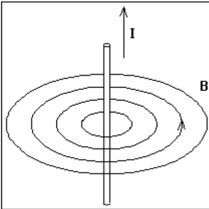
*Fig. 3: Circular Magnetic Field  $B$  around a Conductor Carrying Current  $I$*
