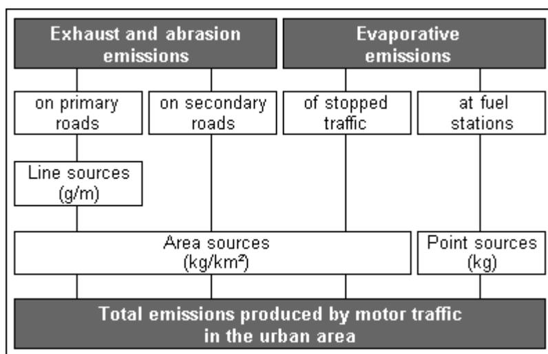
*Fig. 2: Methodology of the 1993 Traffic Emission Cadastre*
