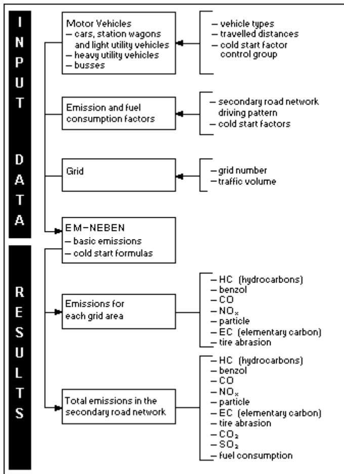
Fig. 4: EM-NEBEN - Emission Model for Secondary Road Network (Area Sources) (Liwicki, Garben 1993)
