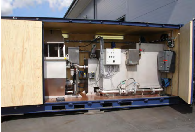
Pilot disk filter facility with microfiltration
